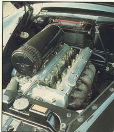
The MkVII has presence, attractive styling and, best of all, the 3,442cc XK twin cam engine from the XK120
